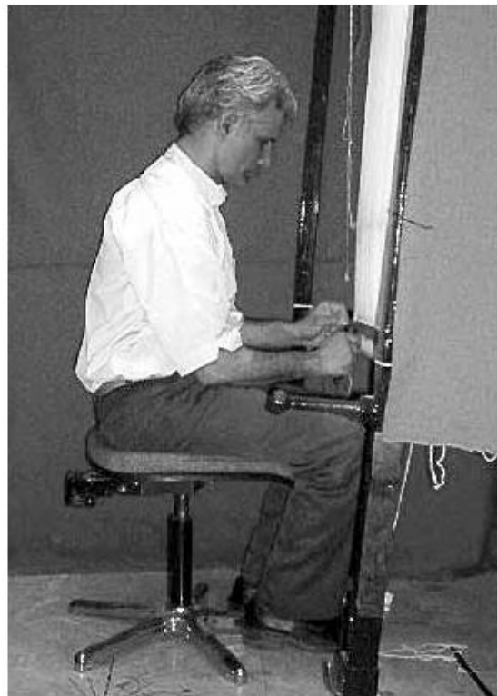
Figure 3. A prototype of the designed loom and workstation. Legs are well supported. There is enough clearance under the loom for legs. The overall body posture is neutral.
